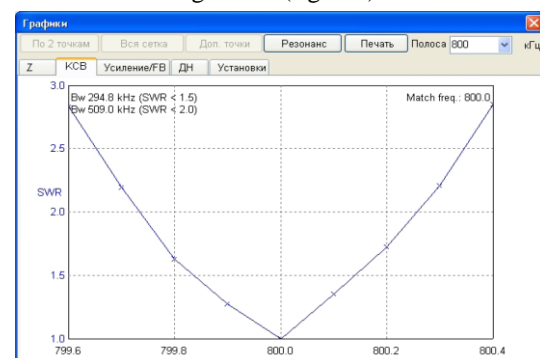
Fig. 10. A amplitude-frequency response (AFR) of meander-line vibrators 10×10 (bandwidth reached 0,06 %), synthesized by means of ACO (fig. 2.b).
