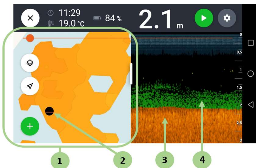
Fig. 3. The interface of the mobile application for working with Deeper PRO: 1 – bottom scanning results; 2 – the current location of the sonar; 3 – bottom structure; 4 – vegetation layer.
